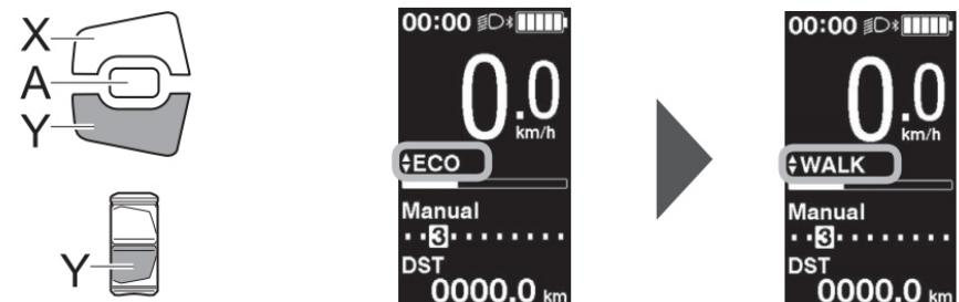
**Warning:** A warning tone will sound while switching is in progress if it is not possible to switch to [WALK] mode because the current speed is not [0 km/h] or there is pressure on the pedals etc.
