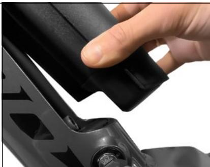
Store the battery in a dry place at a temperature between 5 and 20 °C. The state of charge should be 70 % of the full charge capacity.
