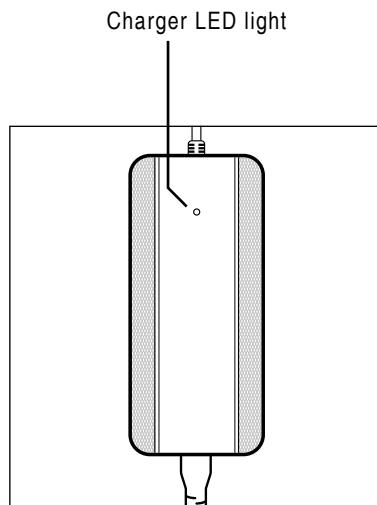
The correct order for connecting the battery to the mains is always to connect the charger to the battery first and then to the mains, otherwise a short-circuit may occur and render components of the E-BIKE unusable. Use only the original charger and lithium battery supplied with the bicycle. Other types of chargers or batteries can cause serious injury or irreversible damage to the bicycle.
