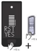
Fig. 10: Resetting to factory settings
