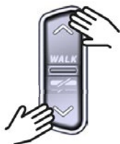
Fig. 6: Selecting the assistance mode in HPR Remote V02
