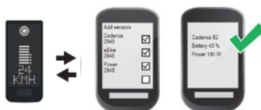
Fig. 8: Connection of the e-bike to the bike computer
